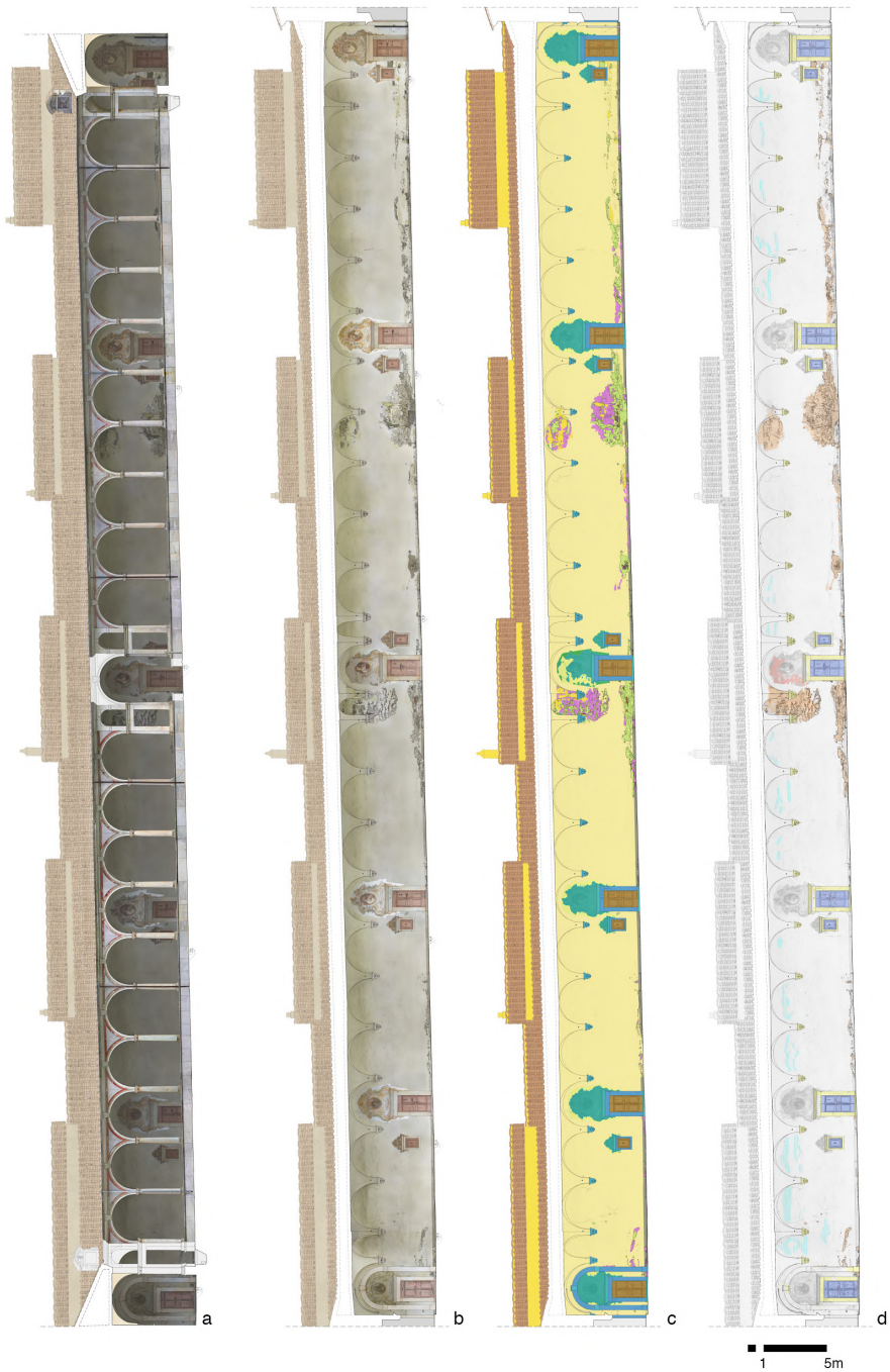
Fig. 2 – Graphic elaborations showing the results of survey activities: a , north external façade; b , current state of the north internal façade; c , material analysis; d , decay mapping (drawing by Giovanni Bruschi and Chiara Gallorini, November 2019).
