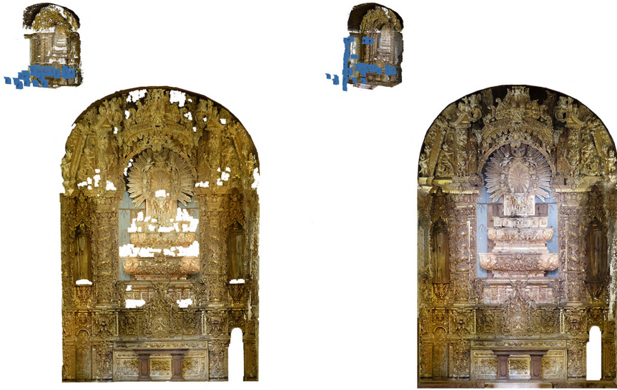
Fig. 10 – Orthographic images exported from the photogrammetric model of the retabulo: reflex acquisition (left), drone and reflex acquisition (right). ©Roberta Ferretti, 2021.
