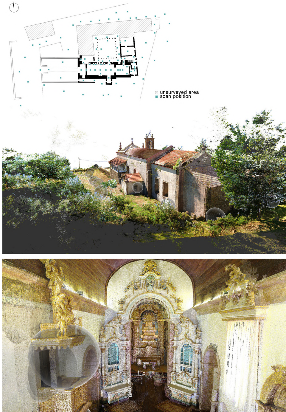
Fig. 7 – Ground floor plan with the position of the scans made with Faro Focus M70 (top). Three-dimensional visualization of the point cloud: exterior view of the convent (middle) and inside view of the church (bottom). ©Roberta Ferretti, 2021.
